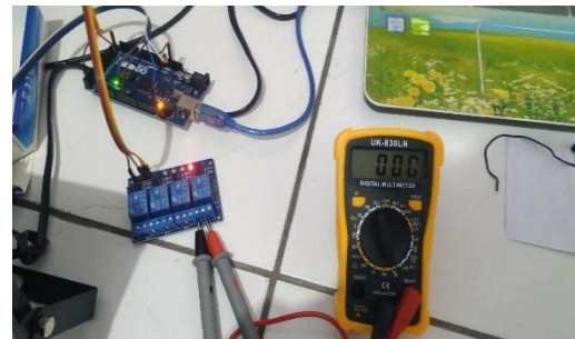
Gambar 9. Pengujian Relay 4 Channel
