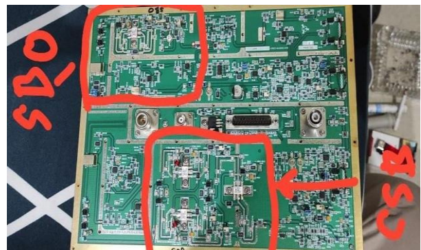
Figure 5. The Power Amplifier Module is in the Checking Process
