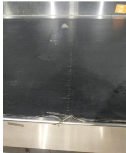
Figure 1. Conveyor belt damage
